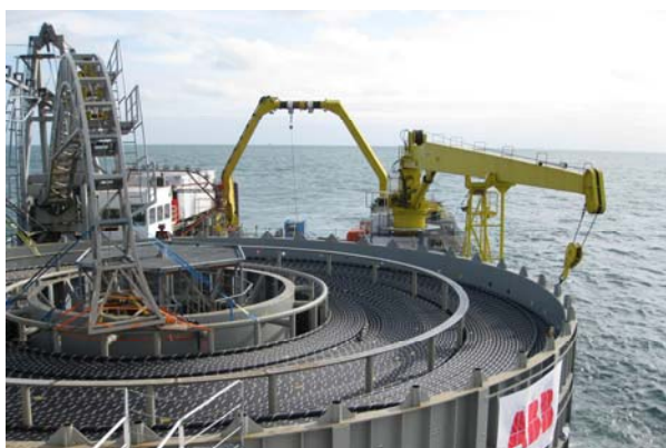
One of Vallvik's special products is a pulp used to insulate advanced power cables. Here, an underwater cable is being laid using a special cable laying vessel.
