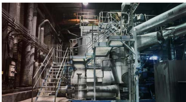
Equipment for the steam pre-treatment of wood chips on the CTMP line at Rottneros Mill. Approximately 25 percent of the raw materials bought in by the Group is in the form of finished wood chips.
