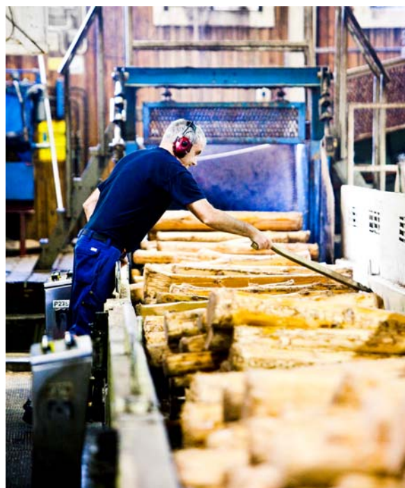
First phase of wood grinding at Rottneros' groundwood line.
