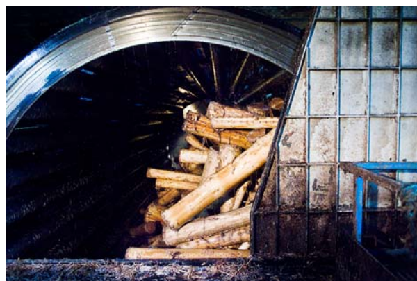
Spruce logs in the debarking drum at the groundwood line at Rottneros Mill.
